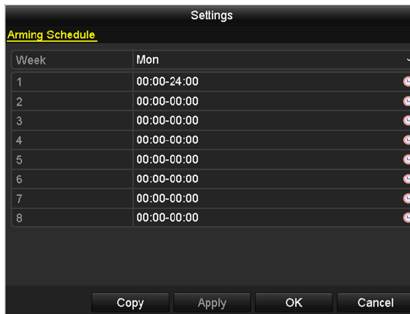
Figure 7-16 Set Arming Schedule of Alarm Output
